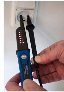
Voltage tester CAT III with low impedance test for detection of ghost voltages
